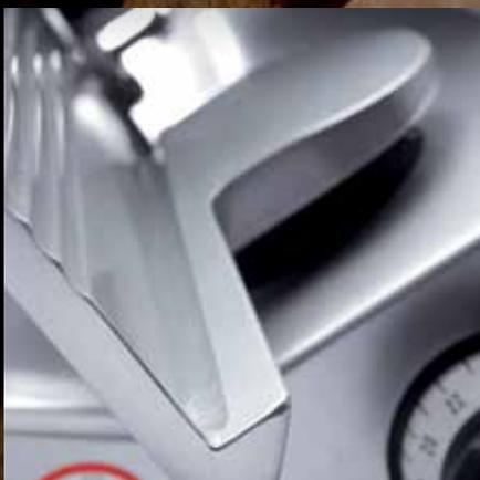
*Drain on gauge plate: reduces the risk of bacterial contamination caused by residual liquids.*
