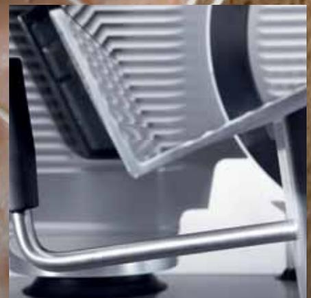
*Carriage handle attached directly to carriage base: no joints mean it is easy to keep the machine hygienically clean.*
