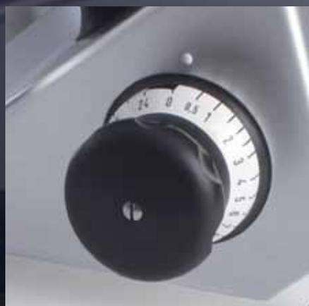
*Rotary knob to adjust thickness with fine adjustment in 0 - 3 mm range: precision slicing and maximum yield for low product residue so far unattained by other competitors.*
