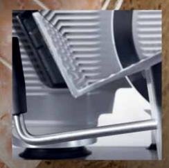
Carriage handle attached directly to carriage base: no joints mean it is easy to keep the machine hygienically clean.
