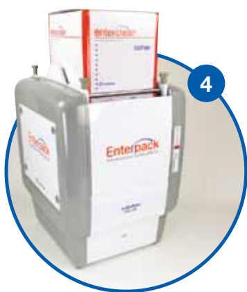
The tray is being sealed and film trimmed
