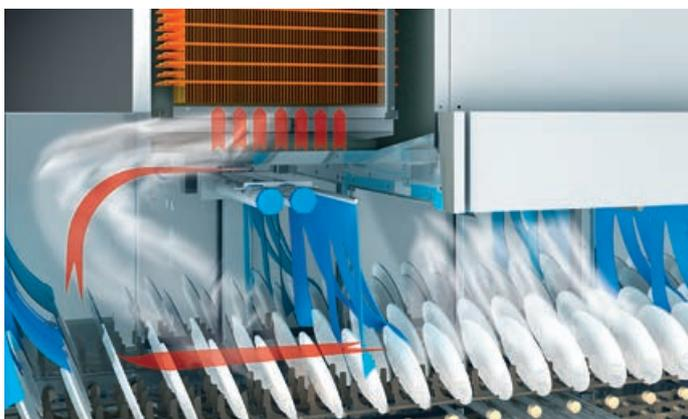
Keeping things cool: The flow of heat is diverted, the hot steam and vapour cool down – and the M-iQ takes the opportunity to gain new dishwashing energy.
