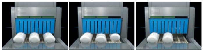
M-iQ *GreenCoach* uses a green indicator light to show which lines should be loaded with dishware at the feed point. This enables the M-iQ to run at optimum capacity at all times.
