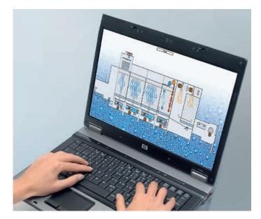
All system-relevant data, functions and operating processes are stored and displayed by the integrated *KMM communication module*. Operating conditions are analysed and diagnosed, and can be easily changed using the computer as necessary.
