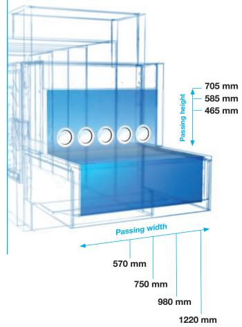
Whether rack type or flight type, the M-iQ fits perfectly with a selection of conveyor dimensions and useful belt widths.
