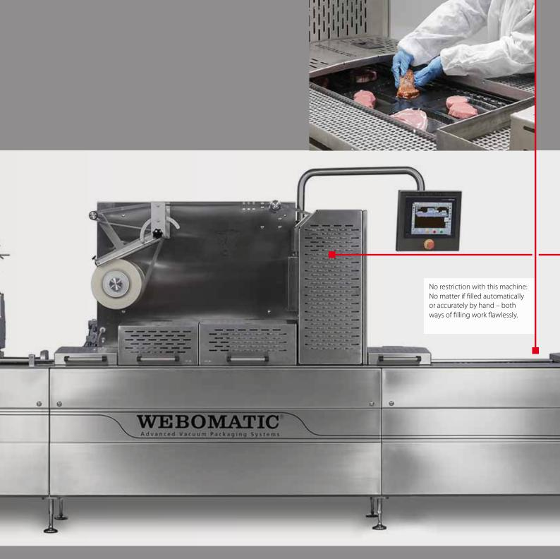
Your product is packed in just a few steps: The film roll feeds the rigid bottom film into the machine and the trays are thermoformed. The packaging moulds car be filled with the product automatically or by hand. In the skin dome, the product is safely sealed. Finally, the punch severs the packs.
